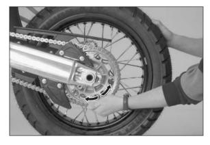
To check the jerk damper: hold the rear wheel while you try to move the rear sprocket back and forth in the running direction.
